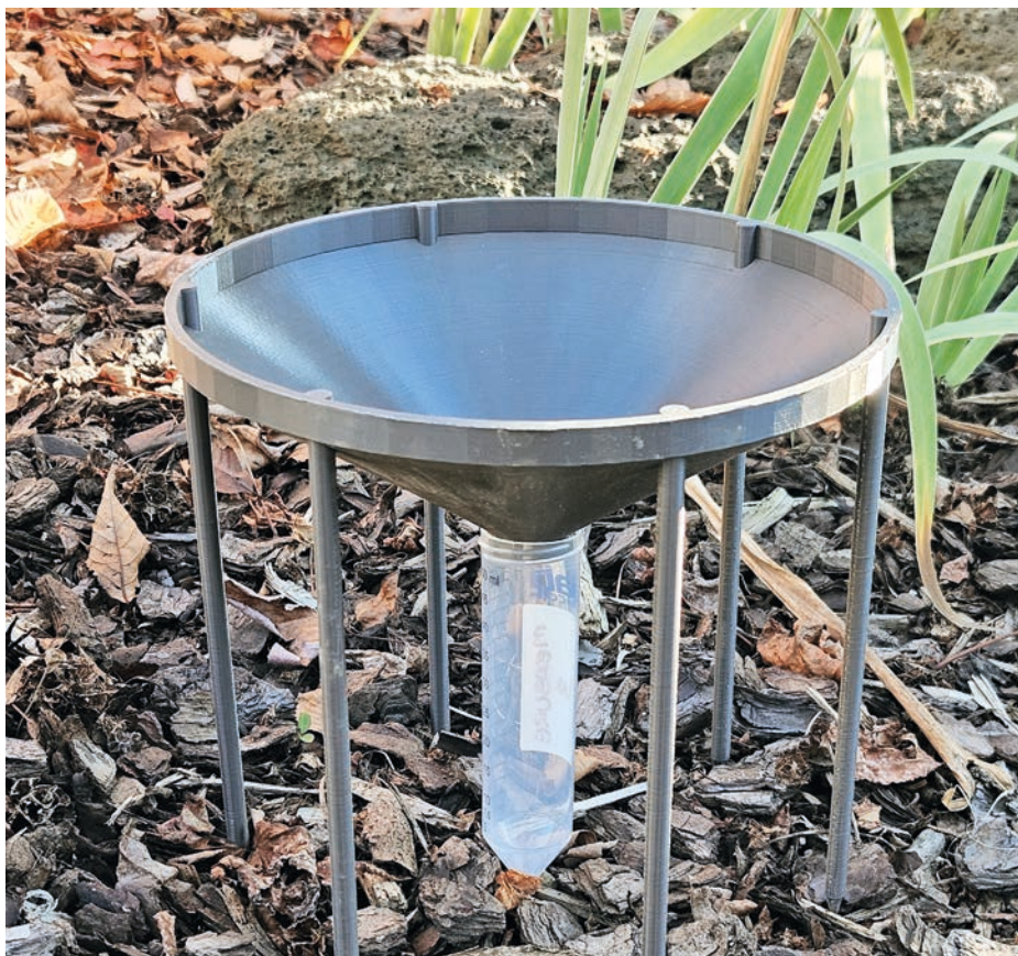
Sample Collection Funnel for Collection of Rainwater for testing.
